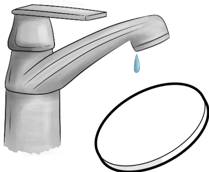
Clean the filters with water and let them dry. The filters must only be reinserted completely dry .
