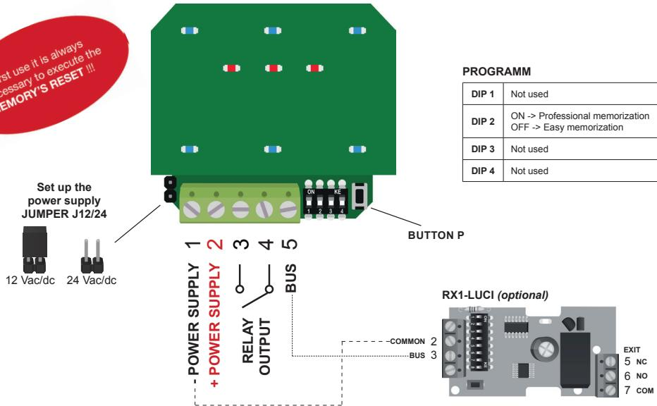
**POWER SUPPLY (1 and 2).** The receiver can me powered with 12/24 ac/dc. If you use direct current respect the polarity (the positive pole in the terminal board no.2)
