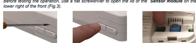
After that step, it is possible to check correct functioning of the LEDs, the BUZZER and the relays by pressing button "A" (Fig.4) or the "TEST" button (Fig.5) as shown below:
