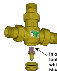
In order to modify the valve setting, it is possible to replace the thermostatic sensor: unscrew the plug, remove the sensor by hand and position the new one.
