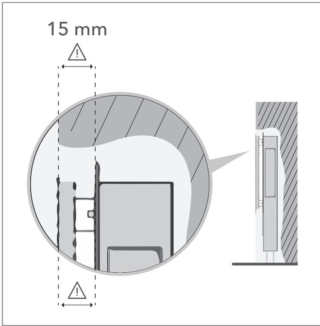
For a correct installation, it is recommended to install the cabinet **15mm deeper in the wall** compared to its overall dimension
